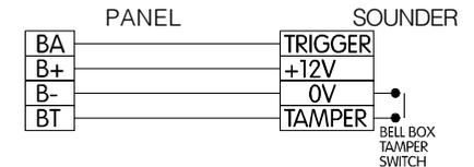
Wiring for mechanical bell:
