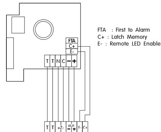
NOTE: C+, E- and FTA connections are all optional. FTA connects to all other PIRs in the same alarm zone. FTA should NOT be connected to the control panel.
