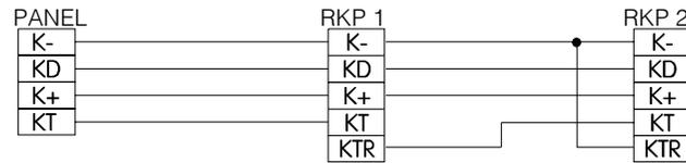
Wiring for multiple remote keypads (star configuration). This requires 5 core cable:
