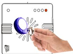
Present the same tag to the reader, and then remove it. The exit time will start on the control panel.
