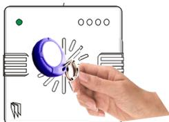
Present the same tag to the reader, and then remove it. The exit time will start on the control panel.
