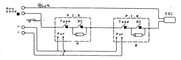
2. WIRING CONTACTS INTO TWO DOUBLE-POLE DETECTION CIRCUITS USING 4-CORE FEED TO CM.DPC MODULE.
