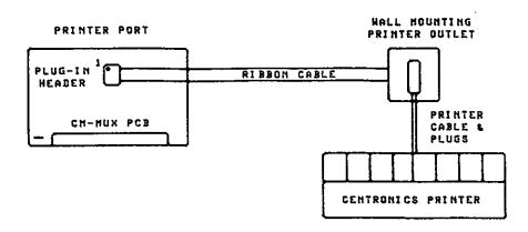
The Omega 8 print facility requires fitting of a CM.MUX PCB. Remove all power to the Omega 8-mains and battery. Plug the CM.MUX onto the lower molex pins on the Omega 8 PCB. ENSURE correct alignment of the pins and that the terminal blocks to the bottom of the panel.
