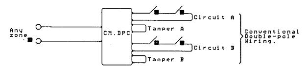
By siting the CM.DPC Junction boxes remote from the panel, a 6-core cable can feed, for example, power (+ and -) and 4 Double-pole detection circuits; OR 6 Double-pole circuits. An 8-core cable could feed up to 8 Double-pole circuits. A simple and effective way of minimizing the number of cables that have to be returned to the Control Panel!! REMEMBER TOO THAT EACH CIRCUIT HAS ITS OWN INDICATION.
