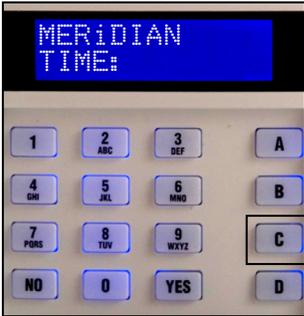
The '**C**' key can be used to select the '**chime**' facility while the system is Unset.
