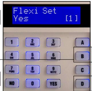
Systems installed to Grade 2 requirements must have 10,000 code differs.
